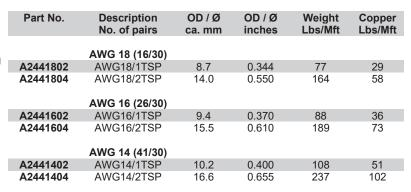
"1000V rated control pair(s) for installation alongside VFD cable. Separating control pairs from the power conductors eliminates ampacity derating otherwise required for composite power cables per 2023 NEC 310.15(C)(1)".
